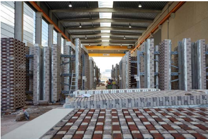
Panels in the factory awaiting transportation to site
