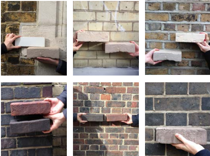
Testing and comparison of brick types against Clerkenwell context brickwork
